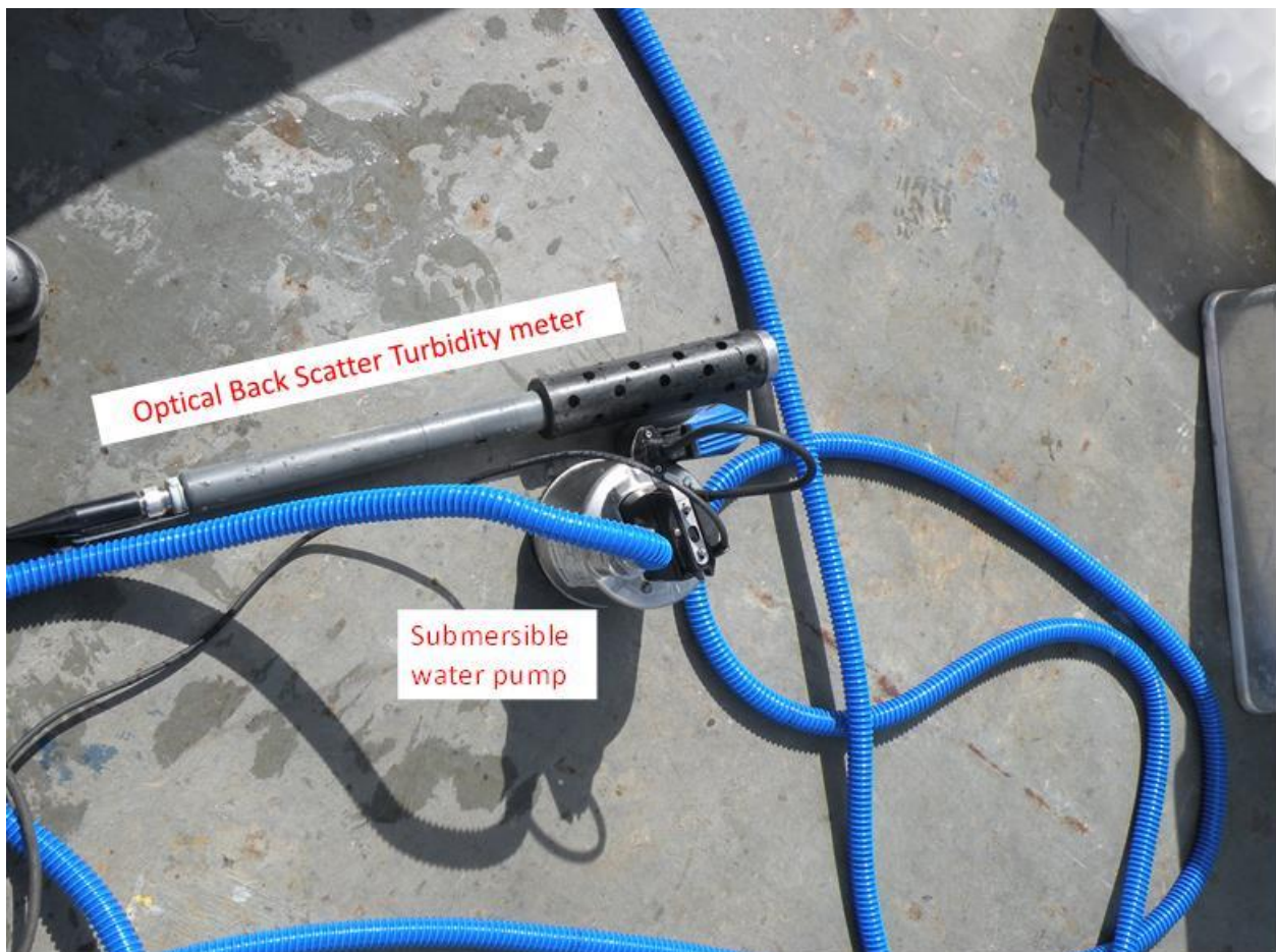
Figure 2: Equipment setup during water sampling
