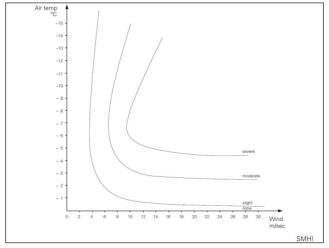
The diagram is applicable to the conditions in the Baltic and the Bay of Bothnia for ships of more than 500 dwt.
