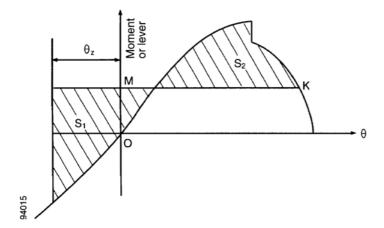
Figure 1 - Static stability curve
