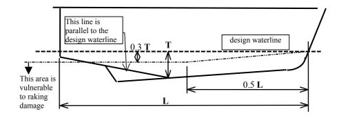
where: T = maximum draught of the hull (each hull considered individually in the case of multihulls) to the design waterline, excluding any non-buoyant structure
