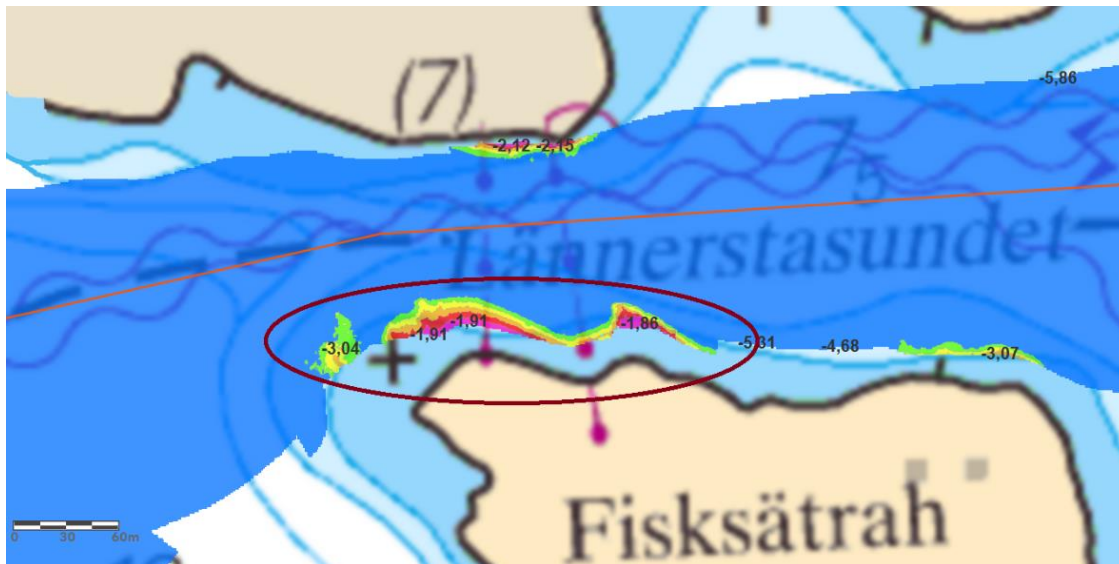
Figure 93. Circled shoals measuring 2 metres outside of the 3-metre curve in the navigational chart were found in Lännerstasundet, north of Fisksätra Holme.
