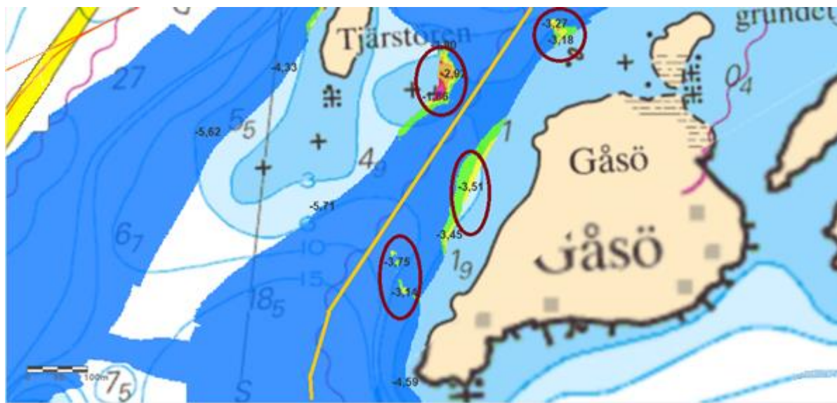
Figure 118. Circled shoals found along the proposed developed route in Tjärstörleden. Proposed route in yellow.
