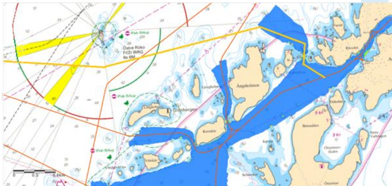
Figure 126. The developed route in corridor 33, the line shown in yellow, is an alternative route for vessels operating corridor 25. The corridor was proposed as the depth through Trålhålet East of Furuklubben was secured by the hydrographical survey.
