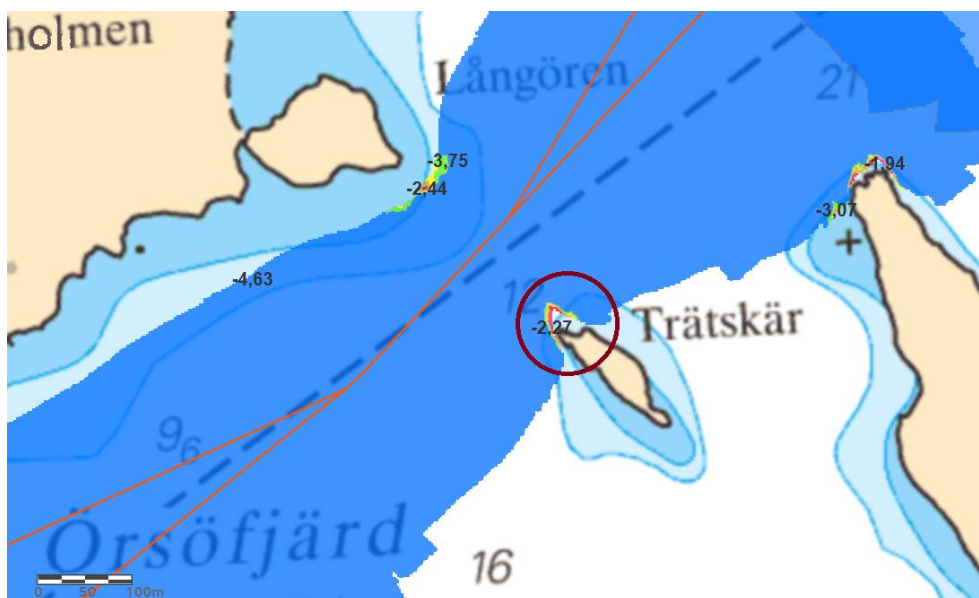
Figure 33. Circled shoal north of Trätskär in Örsöfjärd, causing a safety risk for the ferry traffic.
