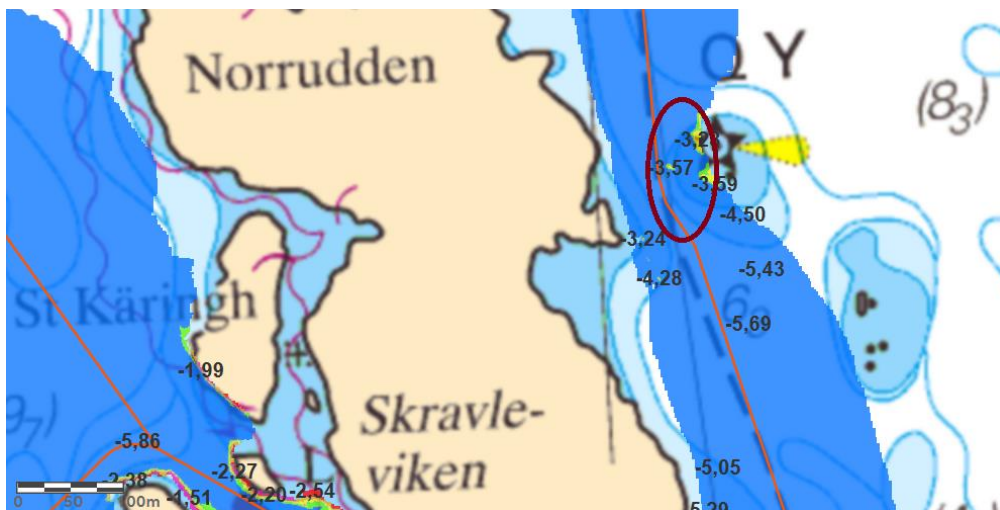
Figure 112. The shoal found at 10-metre deep water according to the navigational chart is circled in the figure. The shoal is situated East of Öja and Norrudden.
