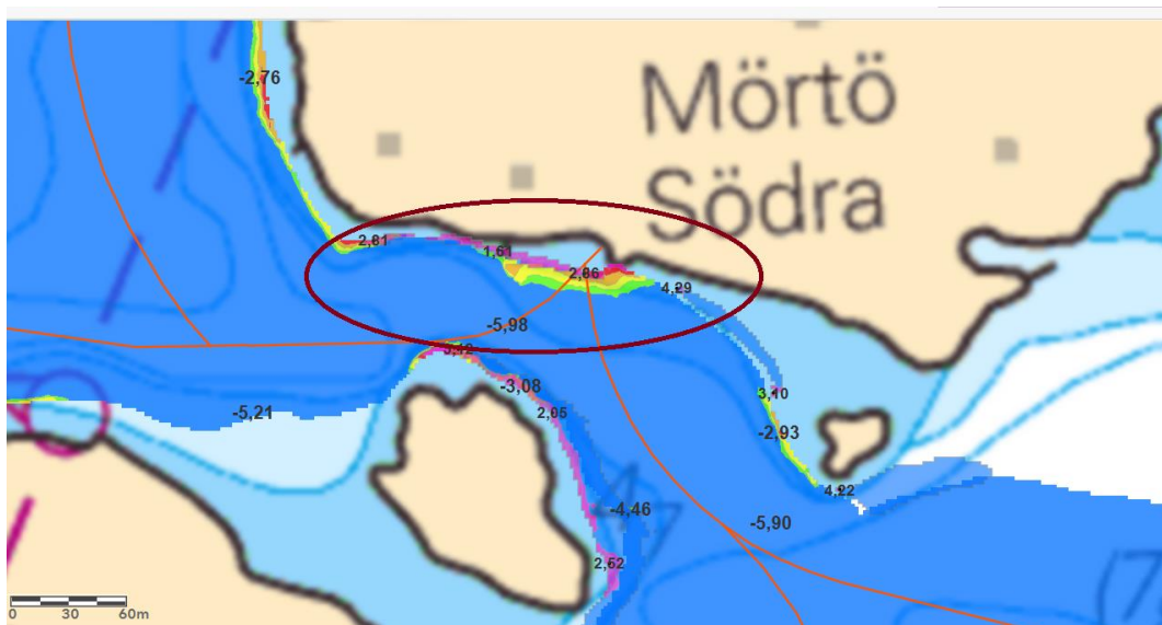
Figure 84. The passage south of Mörtö Södra was found to have a greater depth than known, although, the area around the jetty, circled in the figure was still as shallow as known.
