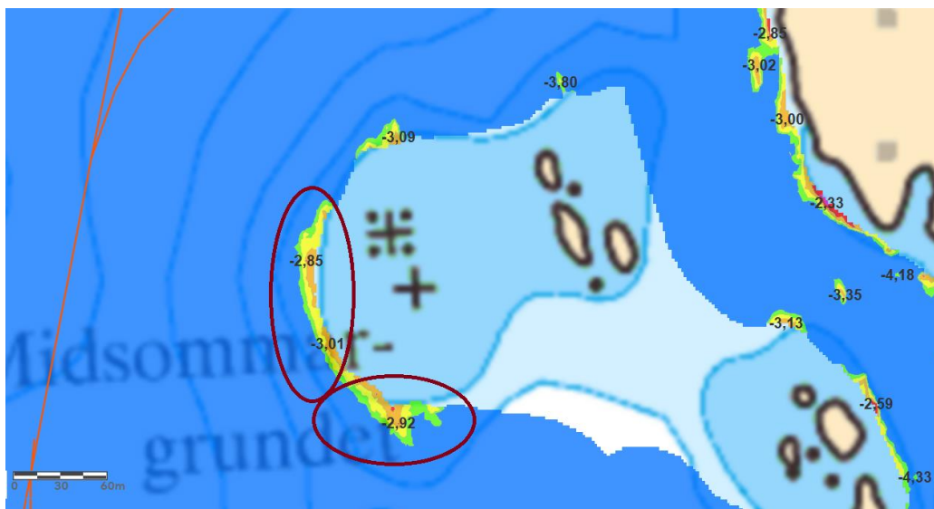
Figure 90. The 3-metre curve on the navigational chart next to Nämddö and south west of Ekholmen is positioned too far in. Shallow areas further out than the curve are circled in the figure.
