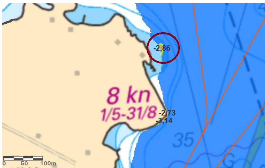
Figure 125. Circled shoal next to Stavsås and north of Tegelhällan in the proposed developed route.
