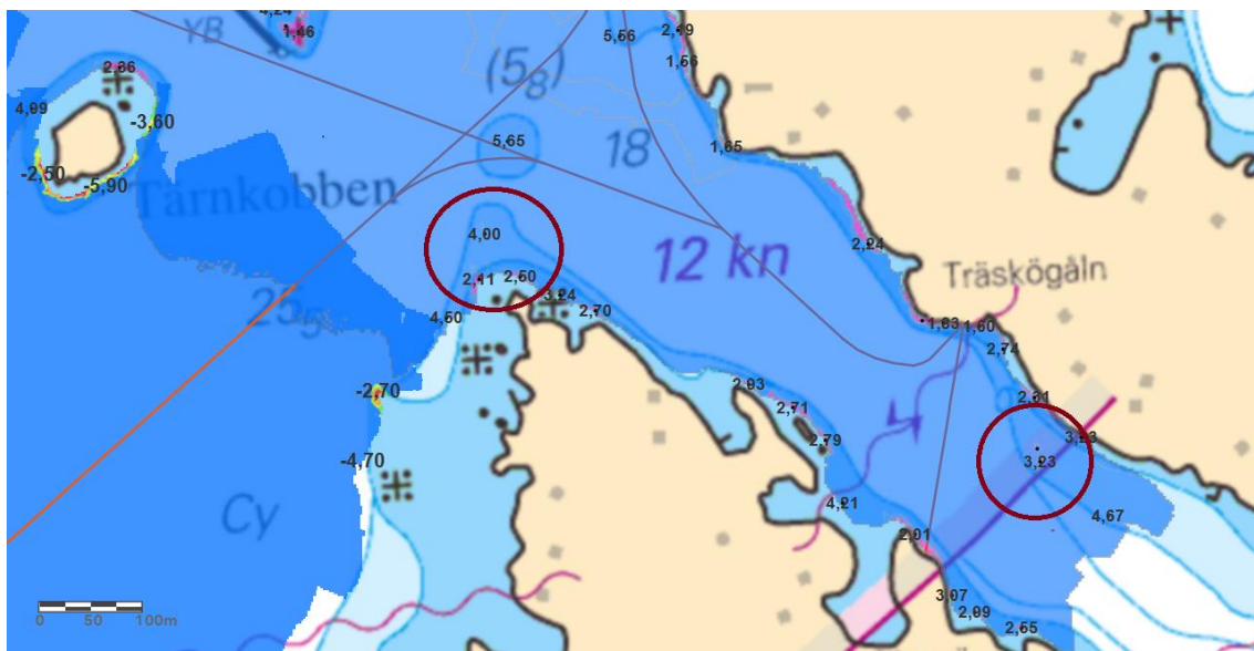
Figure 45. The two shoals close to the jetty of Träskögåln are circled, the circle furthest to the right is also the turning area for the ferries operating the jetty.
