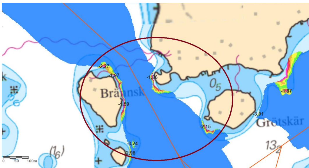
Figure 35. Many locations were shallower than known along the passage between Brännskär and Grötskär, circled in the figure.
