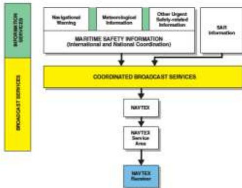
Figure 1 – Basic concept of the NAVTEX system
