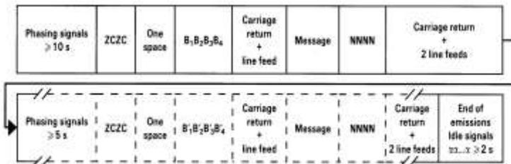
Figure 6 – Standard format for NAVTEX messages
