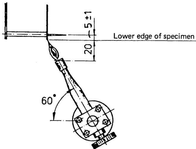
Figure 2 – Ignition burner – Fabric positions
