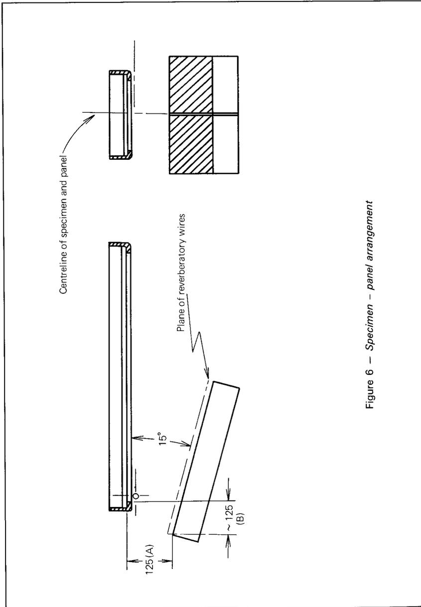
Figure 6 – Specimen – panel arrangement
