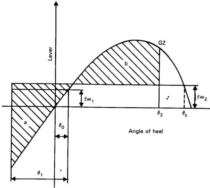
Figure – Severe wind and rolling
