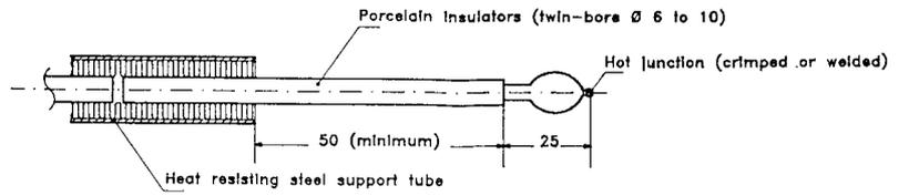
Stainless steel sheathed thermocouple assembly
