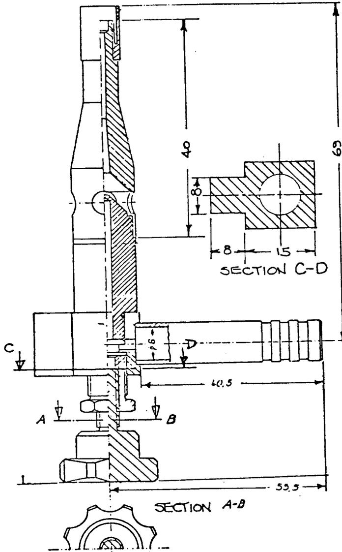
Figure 1 — Ignition burner\*
