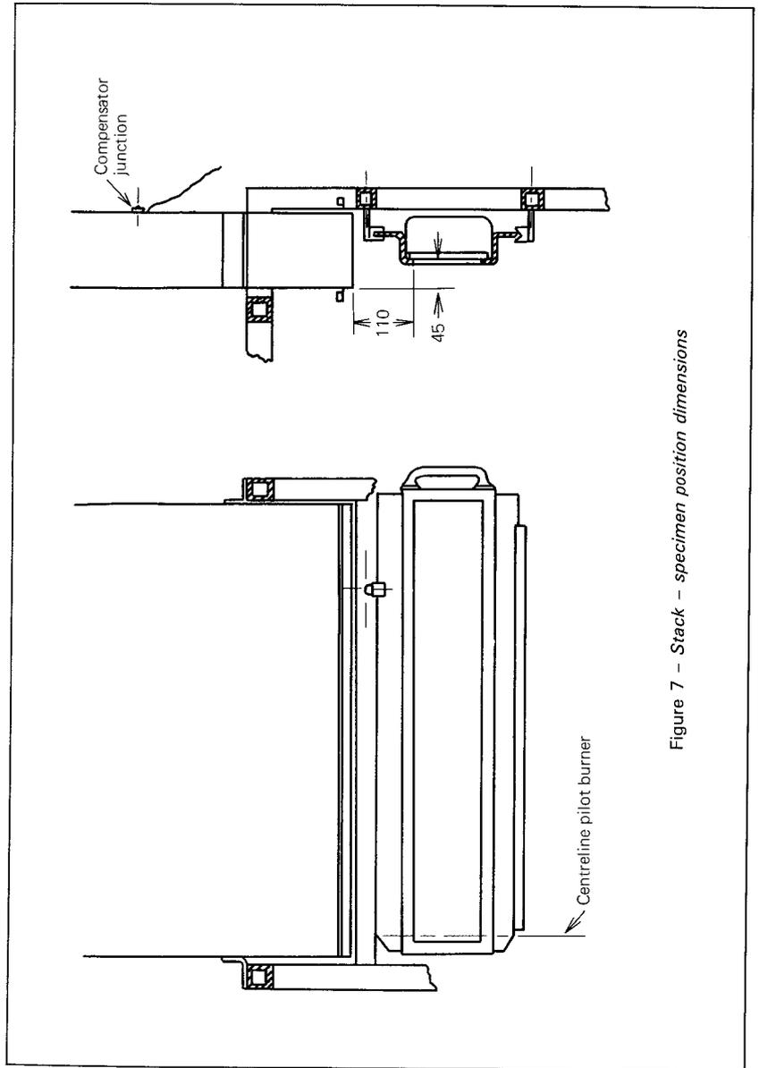
Figure 7 – Stack – specimen position dimensions
