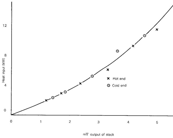
Figure 12 – Typical stack calibration
