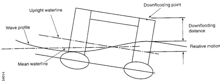
Figure 4.6-4 - Definition of downflooding distance and relative motion
