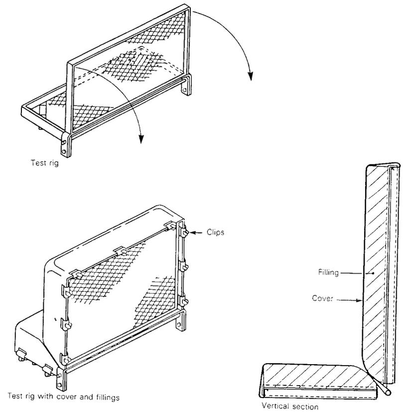
Figure 2 – Test rig assembly
