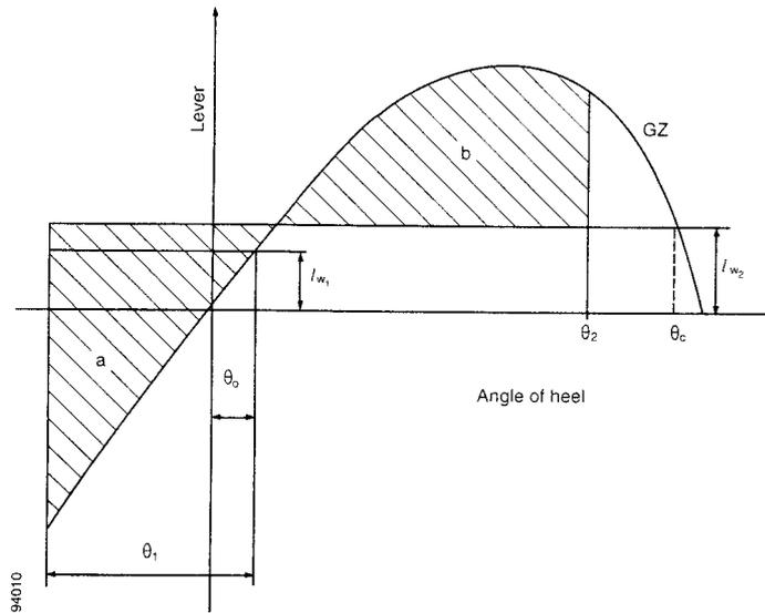
**Figure 3.2.2.1 - Severe wind and rolling**
