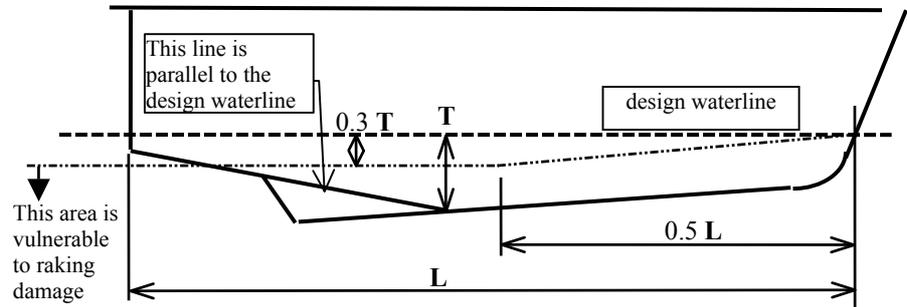
where:  $T$  = maximum draught of the hull (each hull considered individually in the case of multihulls) to the design waterline, excluding any non-buoyant structure
