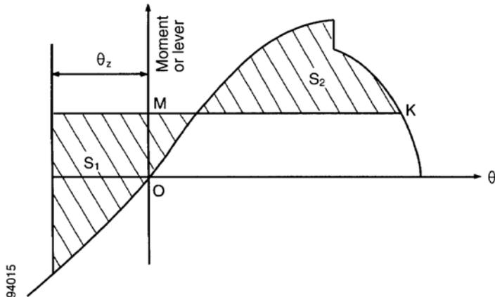
Figure 1 – Static stability curve
