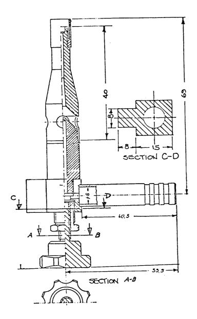
Figure 1 – Ignition burner\*
