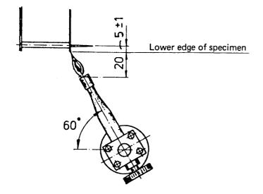
Figure 2 – Ignition burner – Fabric positions
