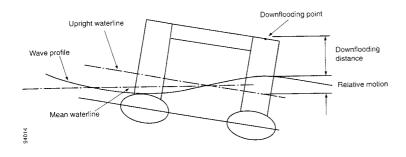
Figure 4.6-4 - Definition of downflooding distance and relative motion
