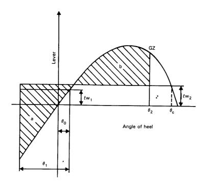
Figure - Severe wind and rolling
