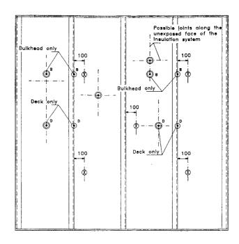
$\bigotimes$  Thermocouples used for maximum temperature rise ' and in calculating average temperature rise
