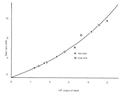
Figure 12 – Typical stack calibration
