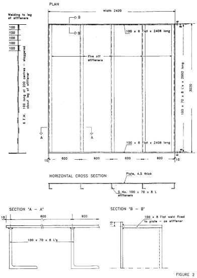
STRUCTURAL STEEL CORE FOR 'A' CLASS DECK AND 'B' CLASS CEILING
