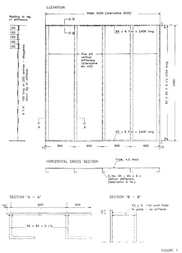
STRUCTURAL STEEL CORE FOR 'A' CLASS BULKHEAD AND 'B' CLASS LINING
