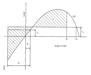
Figure 3.2.2.1 - Severe wind and rolling
