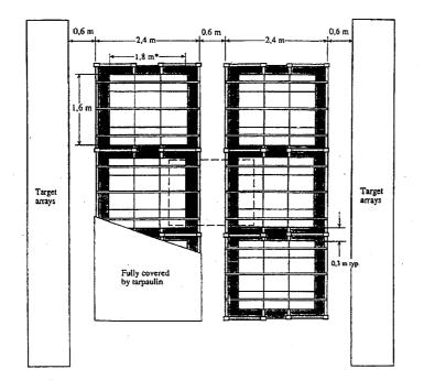
Drawing is shown with EUR Std Plastic sized cartons. \* Should be 1.6 m if FMRC Std Plastic is used. See details of targets in figure 4.
