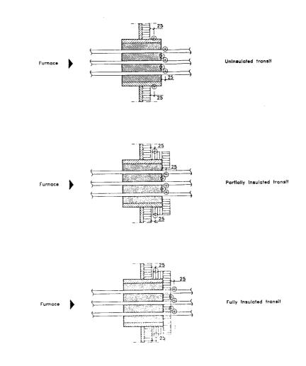
FIGURE AZ CABLE TRANSITS - POSITION OF UNEXPOSED FACE THERMOCOUPLES (SHOWN FOR BULKHEAD)
