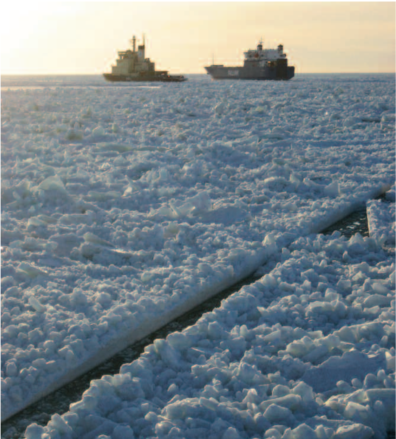
Illustration of the flaw lead and adjoining brash ice barrier that formed in western part of Sea of Åland during March 3 rd - 4 th . Finnish icebreaker SISU can be seen during assistance of a merchant vessel with great difficulties to proceed through the heavy ice drift.
