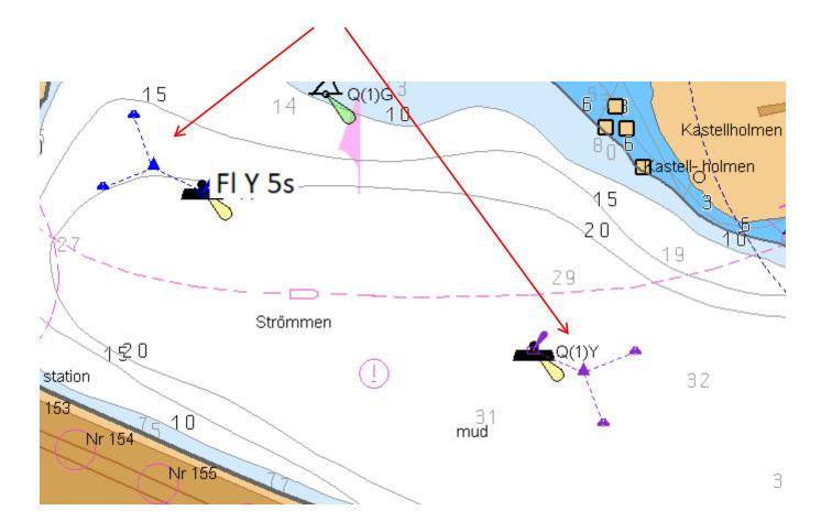
There is ~ 10 m slack in the chain for each buoy which means that the distance between buoys will be ~380m after the lines has been tightened
