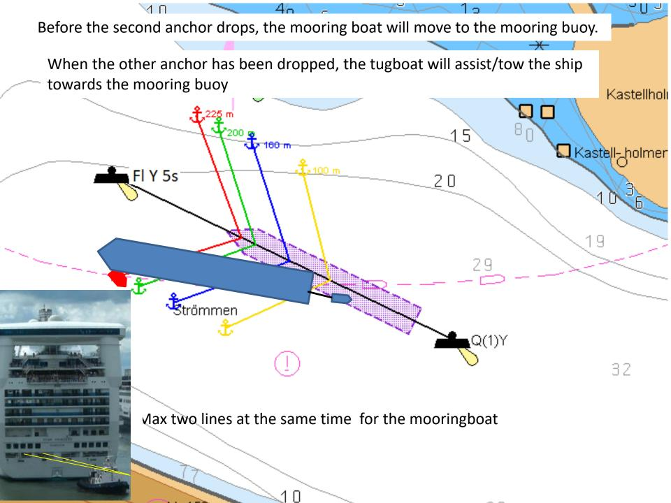
Maximum 6 lines can be used for mooring on the western buoy and 8 lines at the eastern buoy
