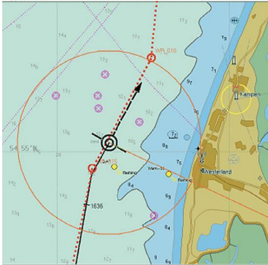
Example of a vector chart with vessel's symbol in the centre
